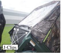
c) Drape the cover over the frames. Attach three J-clips on the front of the dump bed.
