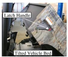
**a**) Tilt the dump bed by pulling the latch handle.
