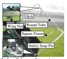
b) Install the two frames into mounting rails, using safety snap pins to secure the square frames. Attached round tube between two square frames. Install bolts on top and wing nuts on the bottom.
