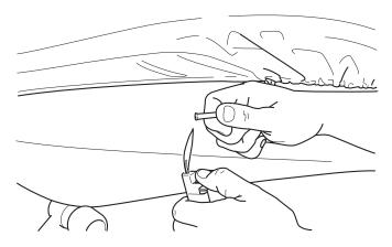
7. Remove the styrofoam plugs from the vacu-vents.
