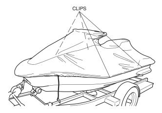
4. Find the knot in the elastic cord located at the front of the cover. Pull the knot and elastic out as far as possible and retie the knot close to the sewn edge of the cover (large enough that it will not slip through the hole).
