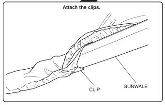
3. Pull the cover completely over the back of the unit one side at a time. Attach all the clips as you go.
