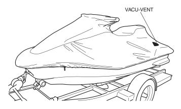
8. To remove the cover, detach the clips, then remove the cover starting at the back of the boat working your way to the front.
