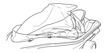
Pull the cover completely over the front of the PWC, until it reaches down under the bow. Attach the clips to the gunwale as shown and make sure they are evenly aligned.
