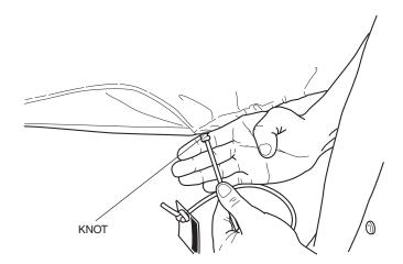
5. Ensure the knot is secure then cut the excess elastic cord.
