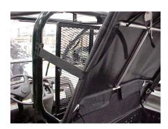
6. Magnet is held in place when not in use by applying to large washer on opposing metal arch in tonneau cover.
