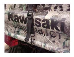
5. Tonneau cover may be held open using supplied magnetic strap by applying to roll bar or other steel portion of cab.
