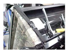
4. Secure rear end of tonneau to vehicle after loading cargo bed by applying hook to the lower rear edge of bed. Tighten snugly by pulling on adjustment strap. Loosen by lifting on bottom edge of plastic slide.
