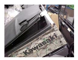
Remove outermost bolt on lower front edge of cargo bed and reinstall with provided buckle strap and stainless steel washer as shown. Repeat this step for both sides of vehicle.
