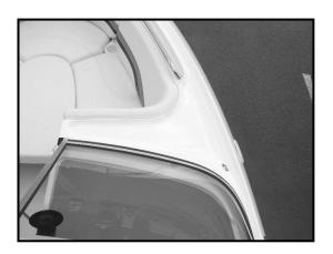
9. The photo to the right shows the location of the starboard (drivers) side Eye Strap mounting location. The Eye Strap mounts 3" forward of the windshield and 2" in from the crest of the deck. Mark the holes as before, and cover with protective masking tape. Using an 11/32" drill bit with a 1/4" drill stop, drill both holes in deck.
