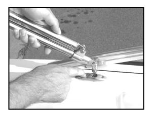
15. The next step is to secure the rear bimini supports into the rear deck hinges. Pin the supports in place when you have them in alignment. See photo to the right.
