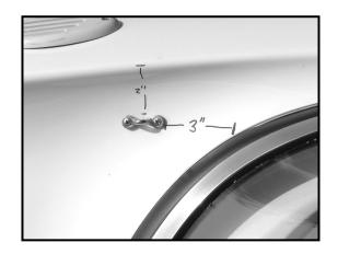
10. After drilling the holes locate the two 8-32 X 1" screws, washers, and nylon lock nuts. These are the smaller diameter screws in the hardware kit.
