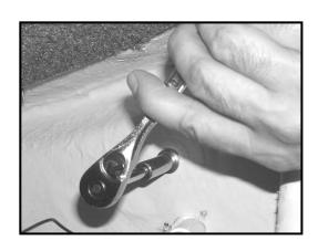
5. Next are the Bimini Hinges. These mount 3 - 1/2" forward of where the wrap around windshield ends. The quick release button should face the stern (rear) of the boat.
