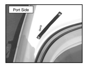
14. With the help of another person, lift the bimini top into place. The main mounts click into the quick release bimini hinges. Once they have clicked in place, try to lift them out to make sure they are securely attached.
