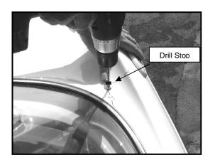
11. You gain access to the back side of the screws on both sides through the right and left storage hatches on the boat. Have a helper hold the Phillips screw on top while tightening the nylon lock nut with an 11/32" socket at 2 foot pounds.
